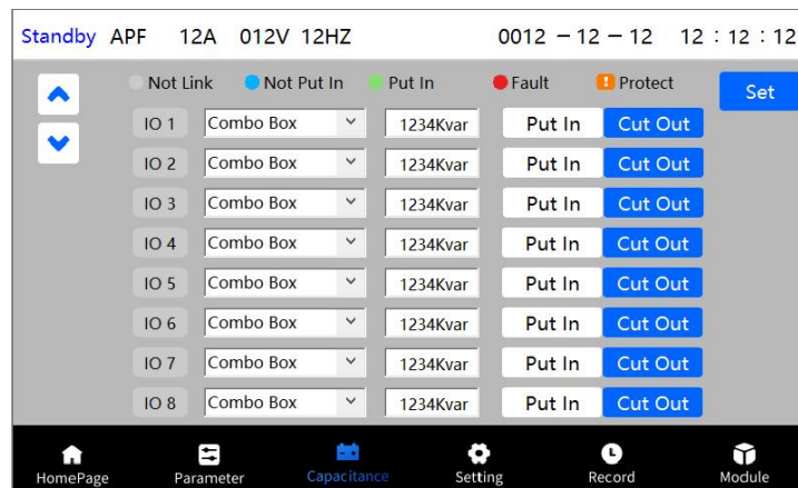
Figure 4.14 Capacitor Switching Interface Second Page
