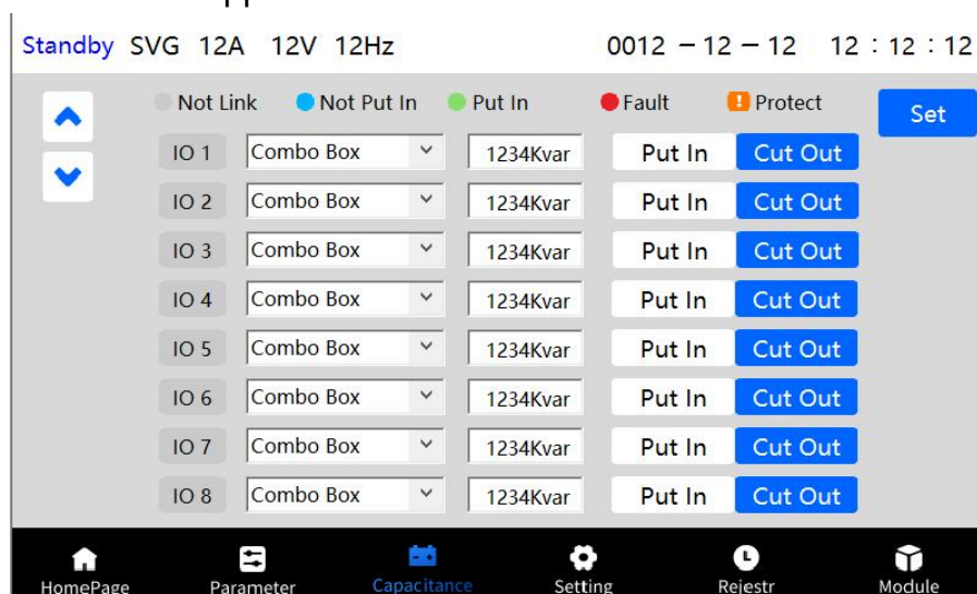
Figure 3-6 Capacitor information interface 1
